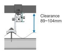
The rail is perpendicular to the rib of roof
